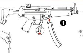
Press the magazine release to remove the magazine. (support the magazine as it may drop.)
