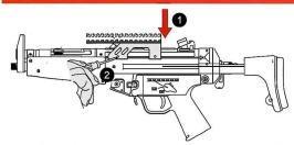
Insert the sight housing from above the gun until it snaps, and then fasten it with a screwdriver. 把瞄准器架從主槍上方,向下扣下 再用螺絲刀擰緊螺絲
